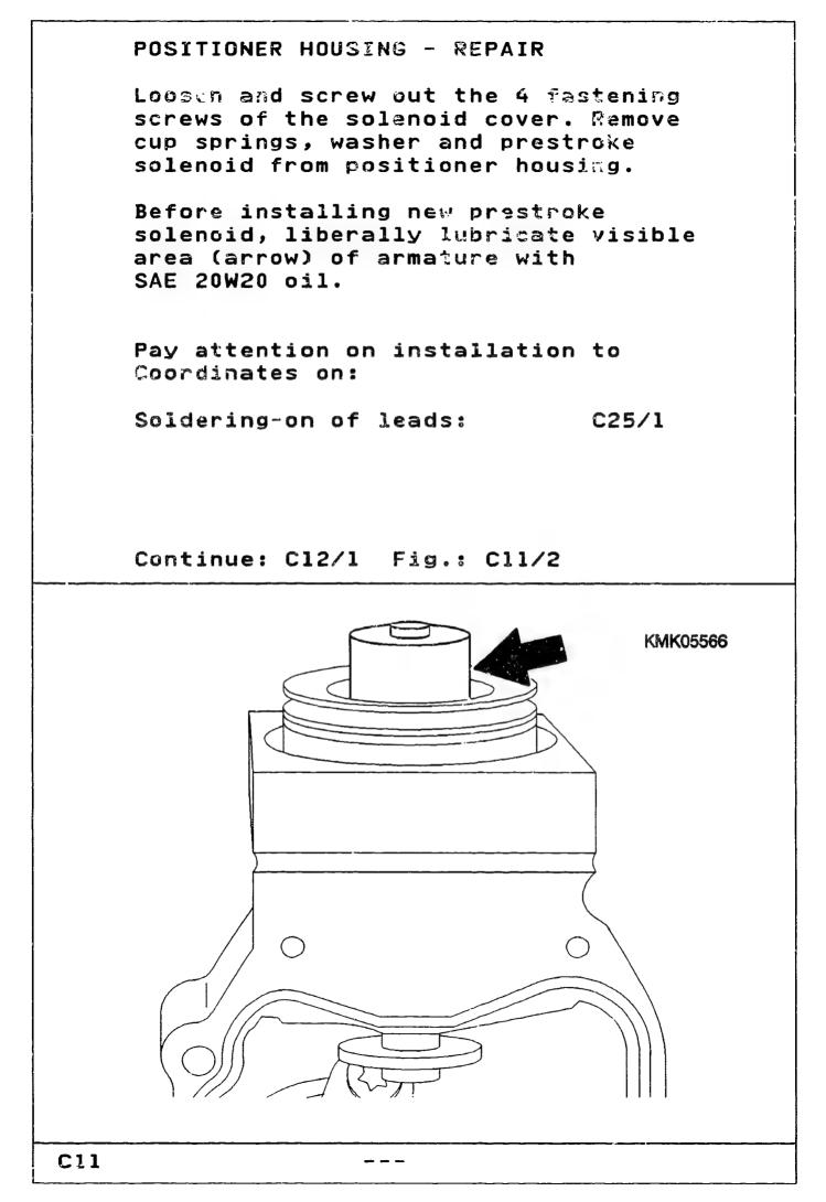
RPS removal - outer plastic seal in positioner housing
